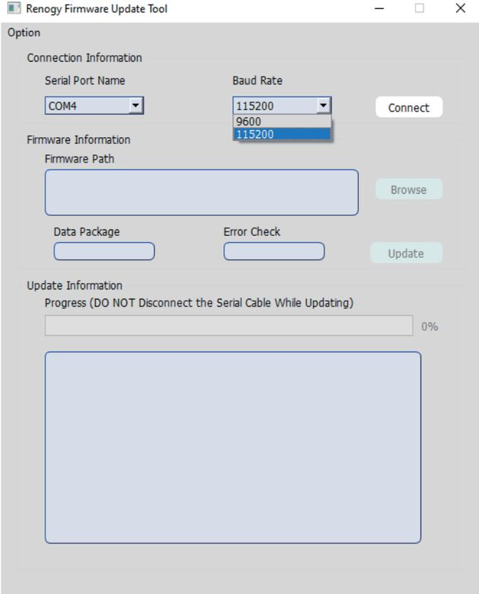
6. Click [Connect] to connect the battery to the Renogy Firmware Update Tool. Once the connection is successful, the current battery firmware version will be displayed in the text box at the bottom of the window.
