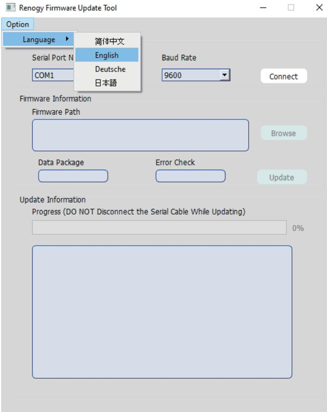
4. Click on the Serial Port Name drop-down menu to select the name of the serial port that the battery is connected to.
