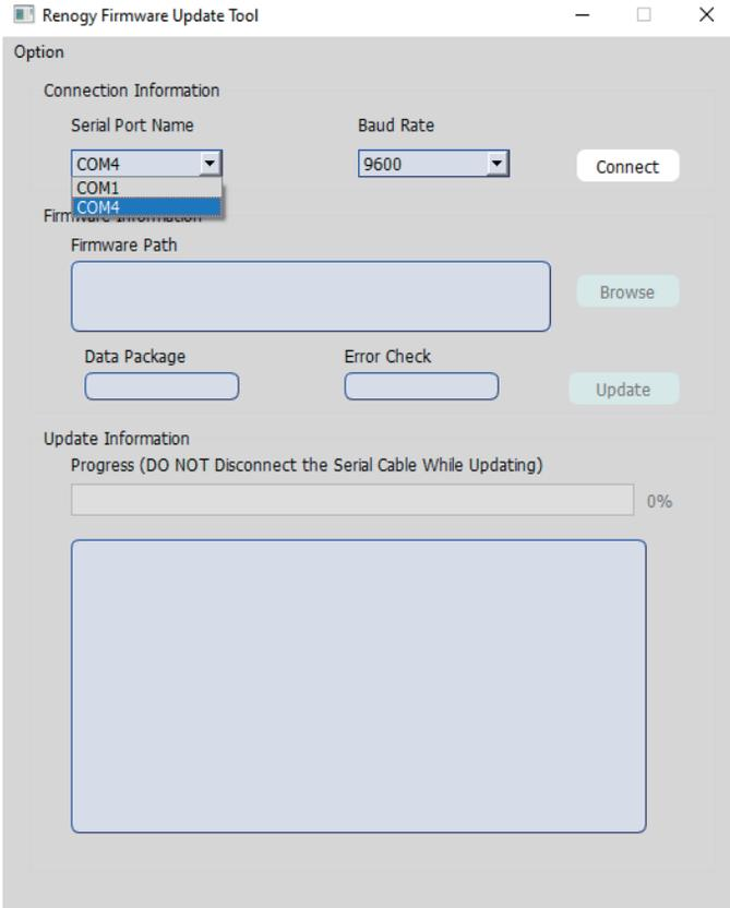
5. Click on the Baud Rate drop-down menu to change the baud rate to 115200.
