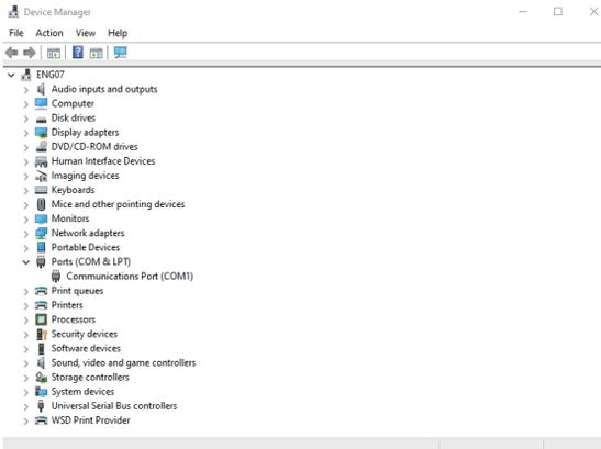
3. Connect the battery to your PC using a serial cable and a new serial port will appear under Ports (COM & LPT), followed by its serial port name.
