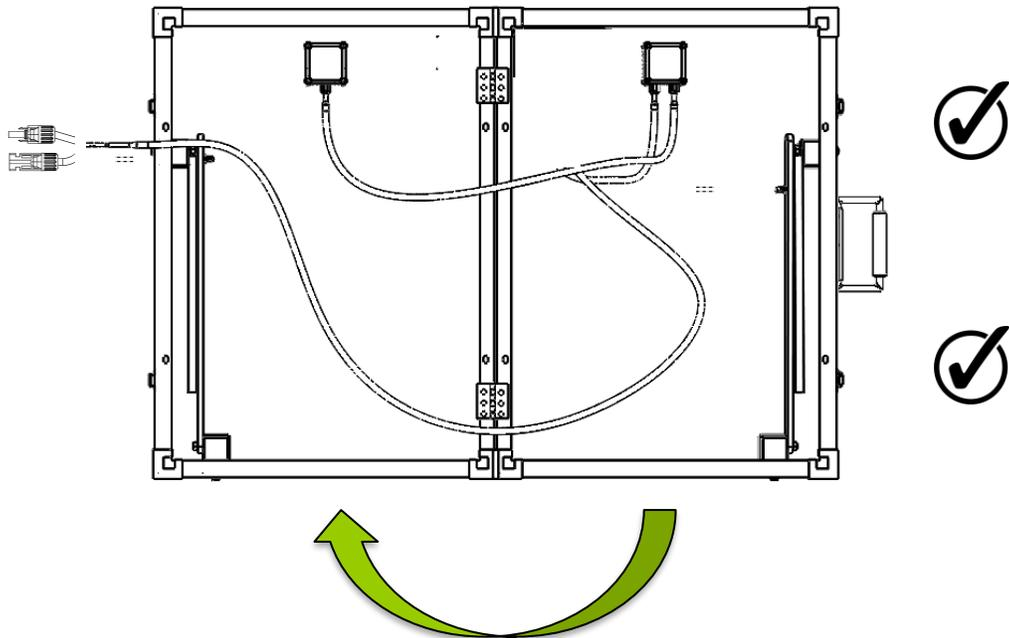
2. Unscrew butterfly nut tilt to desired angle and lock butterfly nut
