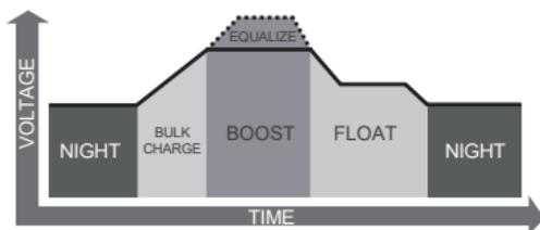
**Bulk Charge:** This algorithm is used for day to day charging. It uses 100% of available solar power to recharge the battery and is equivalent to constant current.
