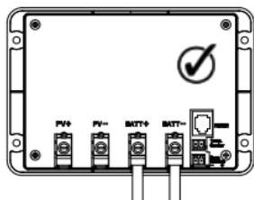
2. Unscrew PV terminals by rotating counterclockwise to open the hatch. Then connect the positive and negative battery connections in their appropriate labeled terminal.
