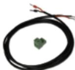
The battery voltage sensor is polarity sensitive and should be used if the adventurer will be installed with longer line runs. In longer runs, due to connection and cable resistance, there can be discrepancies in the voltages at the battery terminals. The BVS will make sure the voltage is always correct to ensure the most efficient charging.
