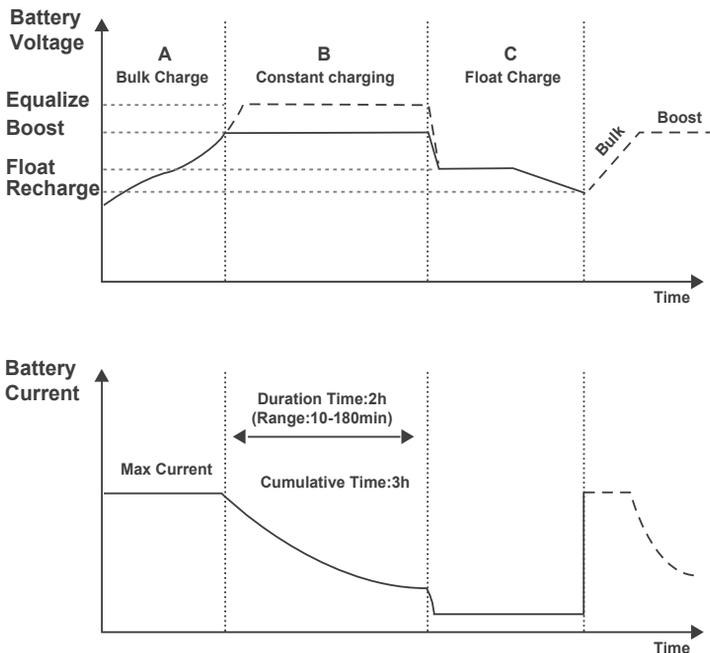
**Bulk Charge:** This algorithm is used for day to day charging. It uses 100% of available solar power to recharge the battery and is equivalent to constant current. In this stage the battery voltage has not yet reached constant voltage (Equalize or Boost), the charger operates in constant current mode, delivering its maximum current to the batteries (MPPT Charging).
